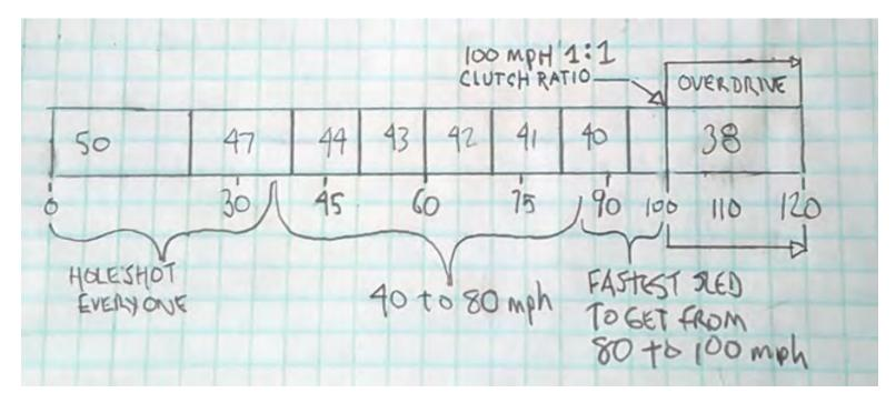
The holeshot broken down to get the sled to speed up hardest to somewhere he had to let off the throttle; this 50/47 degree sped up harder than the stock 47/44.
